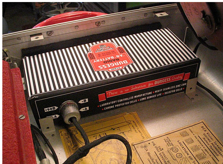
Single AB Battery with 4-pin Connector
