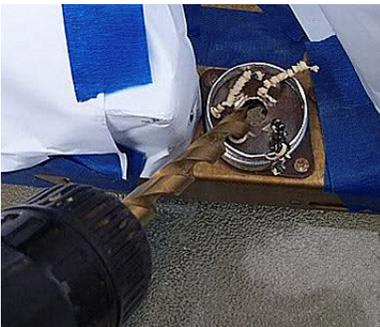
Step 6. Prepare the new capacitors for installation. 60uF, 40uF, and 20uF caps rated at 160 vdc are easy to find. A 22uF cap can be used in place of the 20uF if needed. For the 200uF capacitor, a modern 220uF capacitor rated at 10 volts or more is fine.
