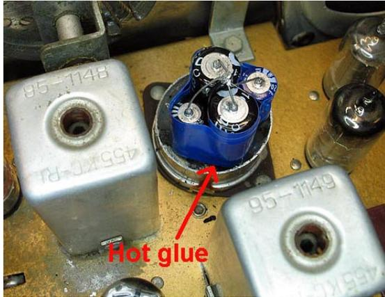
Step 9. Replace the cardboard cover, with the repair facing the dial plate. Re-install the dial. That's it.
