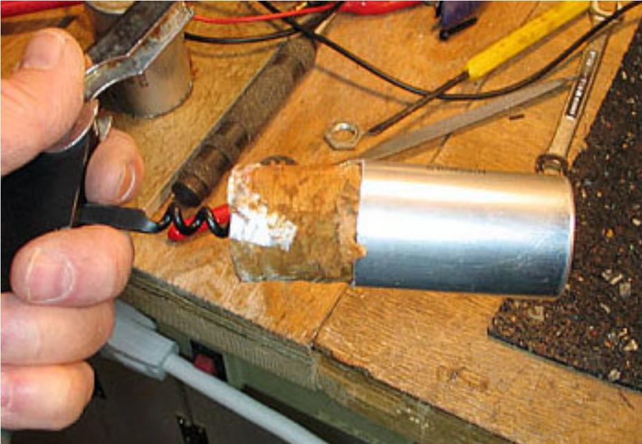
Step 5. Drill a 1/4 " hole down through the center of the bottom part of the multi-capacitor can.
