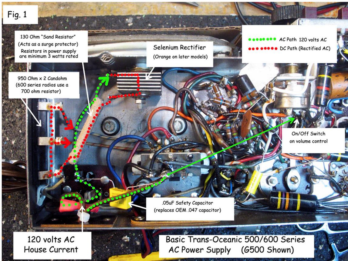
120 volt AC current enters the radio through the power cord. One leg goes to the on/off switch located on the volume control. The other leg goes to the anode terminal on the selenium rectifier. The selenium rectifier removes, or blocks, one half of the AC sine wave, converting AC to DC current, although not a perfect DC current. The electrolytic capacitors filter this rippling DC current to even it out.
