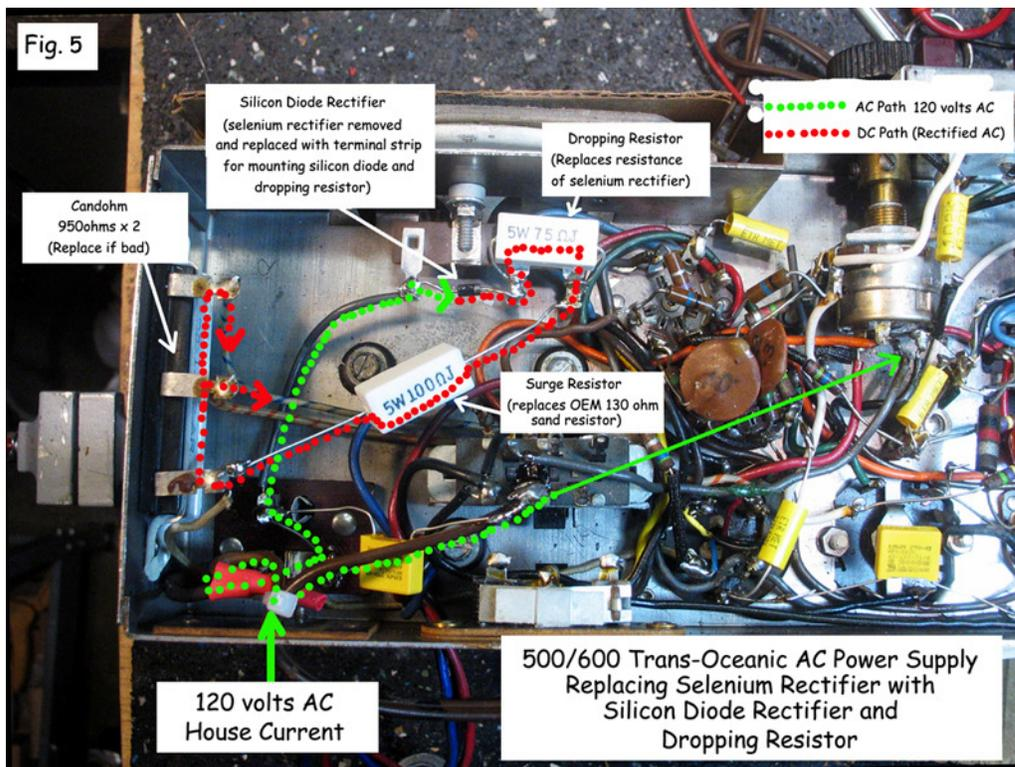
The values shown above are for the specific G500 Trans-Oceanic used as an example. Your values will vary, depending on the condition of your radio and whether you are just replacing the selenium rectifier, or other components in the power supply as well.
