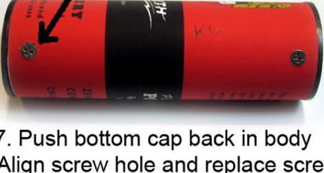
8. Align screw hole and replace screw
