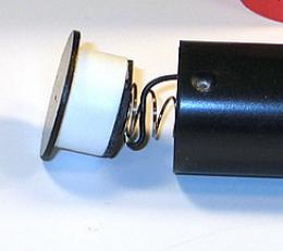
6. Wrap excess black wire around base of spring terminal. Make sure wire does not block contact between battery and terminal
