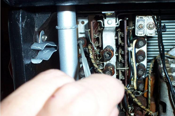
With the 31 meter band tweaked up, it was time to do the 25 meter band. The same procedure was followed. The band switch button was pressed:
