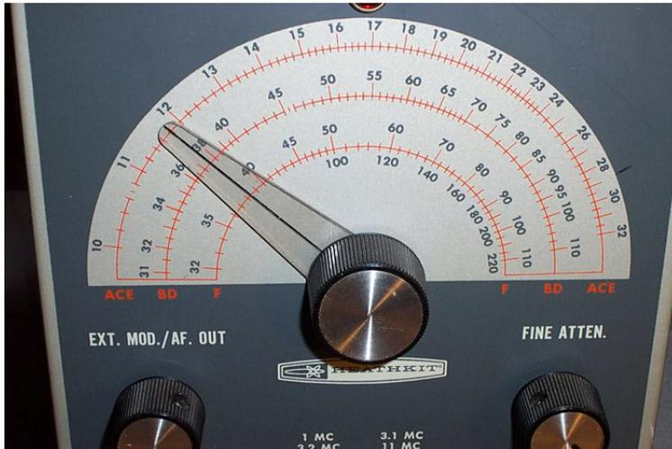
The radio was tuned to 11.8Mc And the second row of coils were tweaked and peaked for maximum signal tone:
