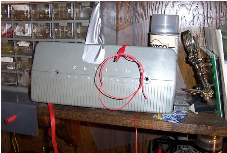
With the signal generator and radio tuned to 1600kc, the oscillator was adjusted for maximum tone (the bottom adjustment screw in the pic). Then the signal generator and radio were retuned to 1400kc and the center screw (RF) and upper screw (Antenna) were adjusted for maximum tone. Each of these adjustments can affect the other, so it's always a good idea to go back and forth two or three times with this until things are peaked out:
